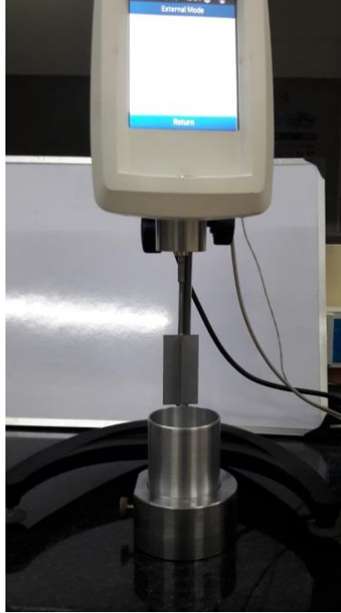
Figure 5.14 Brookfield viscometer with vane test setup (Asphalt Laboratory, IITM)
